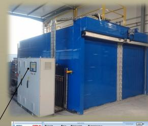
The management of all process parameters is ensured by an in house dedicated SCADA management and supervision software, which provides full traceability and repeatability of the production processes
